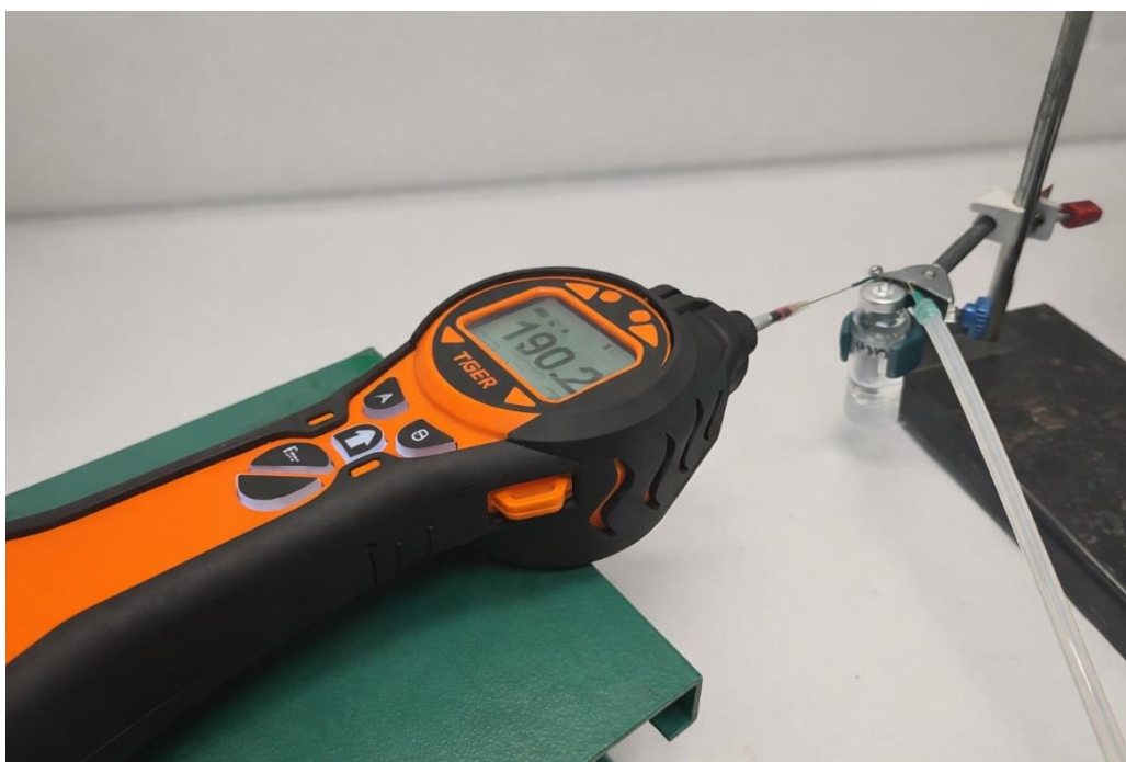
Figure 4.4. PID analyser sampling a test tube, connected with a breather line (at ambient temperature).
